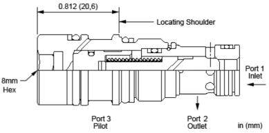
This valve is a spring biased closed, pilot-to-close check cartridge that has a 1.8:1 pilot ratio. The valve allows flow from port 1 to port 2 and blocks reverse flow. Pressure at the pilot port opposes pressure at port 1 at a ratio of 1.8:1. This valve is most often used in regeneration circuits.
