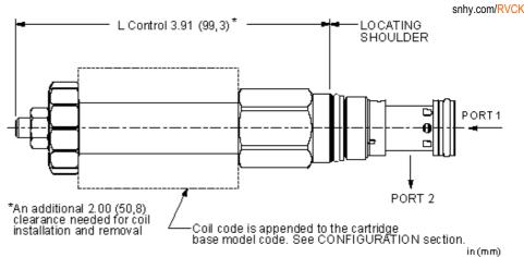
This FLeX Series solenoid-operated, 2-stage, balanced relief cartridge is a pressure regulating valve.
