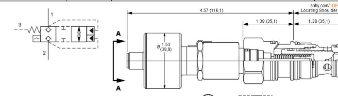
View A-A Pin Diagram These unbalanced, pilot-to-close logic valves are 2-way switching elements that are spring biased closed. Pressure
