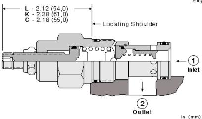
Fast-acting, pilot-operated, balanced piston relief cartridges are normally closed, pressure-limiting valves used to protect hydraulics components from pressure transients. Fast opening and closing is gained at the expense of smoothness. When the pressure at the inlet (port 1) reaches the valve setting, the valve starts to open to tank (port 2), throttling flow to limit the pressure rise. These valves have low pressure rise vs. flow and are very fast.
