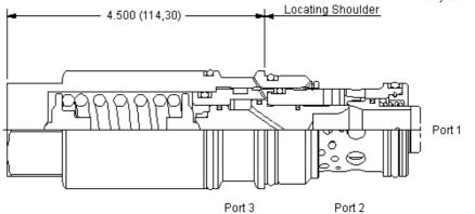
Balanced load control valves combine a balanced modulating element with a reverse flow check. The check valve allows free flow from the directional valve (port 2) to the load (port 1) while the pilot to open modulating element controls flow from port 1 to port 2. Pilot pressure at port 3 determines the flow setting.
