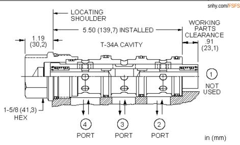
Synchronizing flow divider/combiners are sliding-spool, pressure-compensated devices used to split flow in one direction and combine flow in the opposite direction. With a sychronizing feature, these valves can be used to allow two hydraulic cylinders to fully stroke and synchronize at the end of the stroke. When the first cylinder has reached the end of its stroke, a pressure-compensated, reduced flow is metered to or from the second cylinder until it also reaches the end of its stroke.
