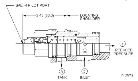
Air-controlled, pilot-operated pressure reducing cartridges use compressed air over a diaphragm instead of an adjustable spring as the setting to reduce a high primary pressure at the inlet (port 2) to a constant reduced pressure at port 1. The air signal is supplied through a port in the hex-end of the cartridge and the hydraulic setting is directly proportional to the air setting at a ratio of 20:1 (hydraulic:air).
