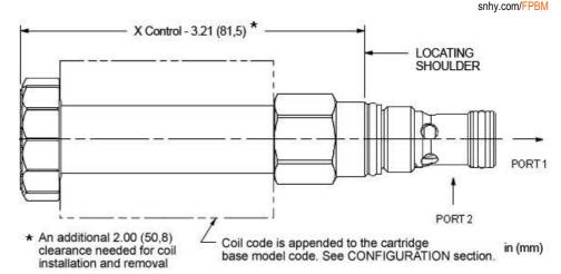
This valve is a pilot-operated, normally open, electro-proportional throttle with reverse free-flow check. Energizing the coil generates a closing force on the pilot stage which pushes the main stage poppet against the seat, proportionally blocking flow from port 2 to 1. In the open condition, flow from 1 to 2 will cause the valve to autoclose and only pilot flow will pass from 1 to 2.
