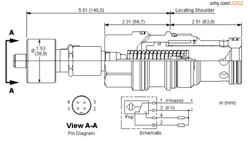
These unbalanced, pilot-to-close logic valves are 2-way switching elements that are spring biased closed. Pressure at either work port 1 or 2 will oppose the spring and tend to open the valve while pressure at port 3 will tend to close it. The force generated by the pressure at port 3, plus the spring force, must be greater than the sum of the forces generated by the pressures at ports 1 and 2 for the valve to remain closed.
