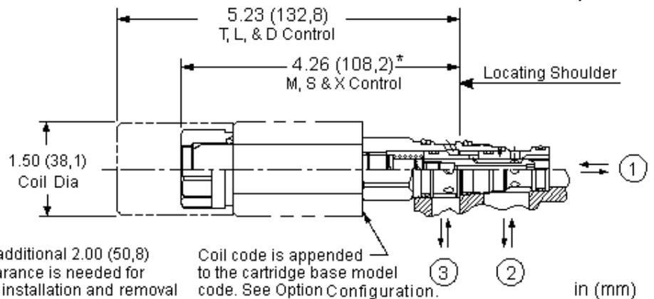
This solenoid-operated 3-way, 2-position cartridge is a direct-acting, balanced spool directional valve.
