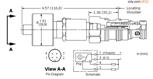
These unbalanced, pilot-to-close logic valves are 2-way switching elements that are spring biased closed. Pressure at either work port 1 or 2 will oppose the spring and tend to open the valve while pressure at port 3 will tend to close it. The force generated by the pressure at port 3, plus the spring force, must be greater than the sum of the forces generated by the pressures at ports 1 and 2 for the valve to remain closed.
