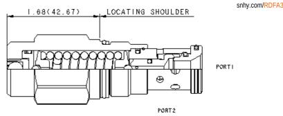
Non-adjustable direct-acting relief cartridges are normally closed, pressure-limiting valves used to protect hydraulic components from pressure transients. When the pressure at the inlet (port 1) reaches the valve setting, the valve starts to open to tank (port 2), throttling flow to limit the pressure rise. These valves are smooth and quiet, essentially zero leak, dirt tolerant, immune to silting and are very fast.
