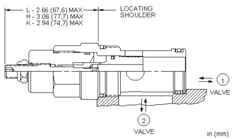
Needle valves are fully adjustable orifices used to regulate flow. They are infinitely adjustable from fully closed up to the maximum orifice diameter. They are not pressure compensated and may be used as flow controls or as shutoff valves.
