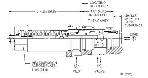
Load reactive, load control valves with pilot assist combine two valves; a check valve and a relief valve. The check valve allows free flow from the directional valve (port 2) to the load (port 1) while a direct-acting, pilot-assisted relief valve controls flow from port 1 to port 2. Pilot assist at port 3 lowers the effective setting of the relief valve at a rate determined by the pilot ratio.
