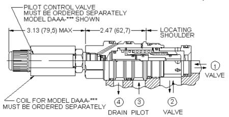
This is a normally open, balanced poppet, switching element with an integral T-8A control cavity. With a 2-way valve in the closed position installed in the T-8A control cavity, the poppet remains open. Opening the 2-way valve shifts the poppet to the closed position, provided there is sufficient pressure at port 3.
