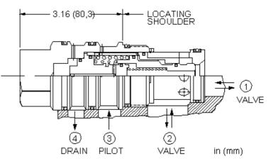
This is a normally closed, balanced poppet, switching element. When the vent port (port 4) is blocked, the poppet remains in the closed position. Venting port 4 shifts it to the open position, provided there is sufficient pressure at port 3.
