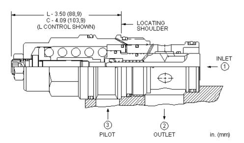
Counterbalance valves with pilot assist are meant to control an overrunning load. The check valve allows free flow from the directional valve (port 2) to the load (port 1) while a direct-acting, pilot-assisted relief valve controls flow from port 1 to port 2. Pilot assist at port 3 lowers the effective setting of the relief valve at a rate determined by the pilot ratio.
